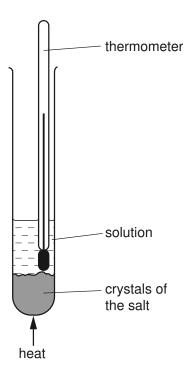
10 g of water was put into a boiling tube. To this  $0.5\,\mathrm{g}$  of potassium chlorate(V) was added. The tube and its contents were heated until the solid dissolved. The tube was allowed to cool. At the first sign of solid appearing the temperature was taken. The experiment was repeated using  $1.0, 2.0, 3.0, \mathrm{and}\ 4.0\,\mathrm{g}$  of potassium chlorate(V).
