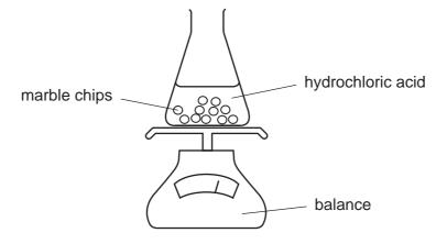
The mass of flask and contents is measured at regular time intervals.
