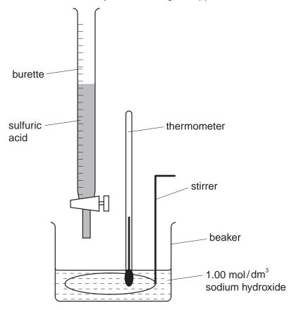
20.0 cm<sup>3</sup> of 1.00 mol/dm<sup>3</sup> sodium hydroxide was poured into a beaker. The temperature of both this solution and the sulfuric acid was 25°C.
