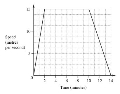
The diagram shows the speed-time graph of a train journey between two stations. The train accelerates for two minutes, travels at a constant maximum speed, then slows to a stop.
